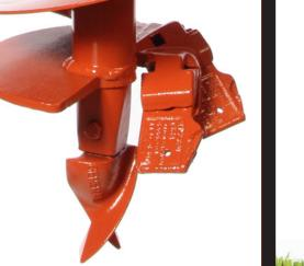
• Field replaceable, alloy steel screw bit, heat treated to extend service life. SB26 screw bit secured with 1 inch square drive lug. Available for specific diameters. • One piece, cast steel LDBH Series boring head design sets tooth position for optimum digging performance. Available for specific diameters.
