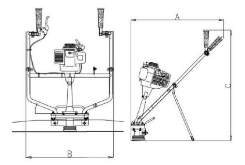
**Hand-Arm vibration** Specification (According to ISO 5394, EN 1033 and EN500-4):  $7.8m/s_2$
