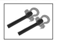
Lewis Pins are used to lift large stones with a crain, chain block or winch. The pins are inserted into specially prepared holes, or seated, in the top of stone directly above its center of mass. Pins are liable to slip out of the seating if some of the weight of the stone becomes in-balanced. For this reason, a safety sling should always be used together with the Lewis Pins.
