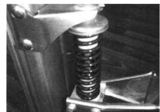
4. The clamp brackets (H31) beside the tube clamps are used to keep the balance of the stilts.
