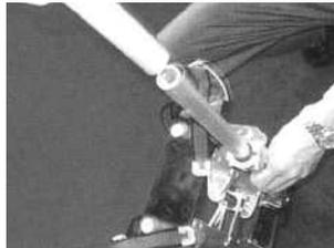
6. Position the tube clamps in the clamp bracket slots, according to your calf size, so the stilts will stand straight when mounted, and tighten them well.
