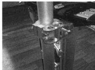
5. Slide the upper strut tubes (H5) down over the lower strut tubes and through the tube clamps. Position so the leg bands (H4) are just above the large portion of the leg calves.
