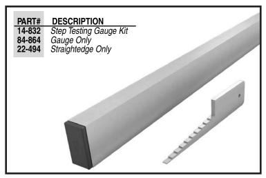
along the straightedge. Deduct one point for each step the gauge is inserted.
