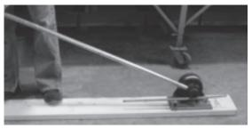
Position your rebar to desired length and then exert enough downward pressure on the handle (kev #8).
