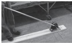
3. While standing on the board (key #9) exert sufficient downward pressure on the handle (key #8) to cut the rebar.
