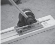
Line up the bending arm so that it is in its lowest position (parallel to the roller (key #11)), and then slide the rebar on the roller and into the bending arm.
