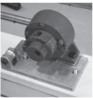
2. Attach the complete housing unit and base casting to the board (key #9) by inserting the 1/2" carriage bolts (key #15) into the bottom of the board. Place the base casting and housing on top of the board and carriage bolts (be sure that neither edge of the base casting is flush with the edge of the board).
