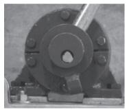
Unit is equipped with 3/4" opening which will cut up to 5/8" rebar.
