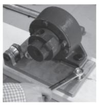
3. Next place the 1/2" flat washer (key #16) and 1/2" nut (key #17) on the carriage bolt and then tighten the 1/2" nut.
