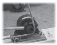
3. In order to make tighter bends remove handle from one socket and position in another socket and continue to bend rebar.
