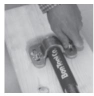
6. For easy storage of Bon's Rebar Cutter/Bender place the steel bar into a socket on the housing unit, and pull the handle down until it hits the board (key #9). Move the handle clip (key #5) over the end of the 54" steel handle and tighten the handle clip down with the 1/4" wing nuts (key #20).
