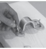
4. To attach the handle clip (key #5) to the board line up the slots on the handle clip with the holes in the board. Insert the 1/4" carriage bolt (key #18) from the bottom of the board and through the handle clip. Then place the 1/4" flat washer (key #19) and 1/4" wing nut (key #20) on the carriage bolt and tighten the 1/4" wing nut.
