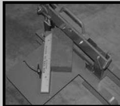
3. If the bottom blade is not touching the brick, adjust the bottom base spring height by tightening down both Bottom Base Hex Bolts until the table height is equal to the bottom blade.
