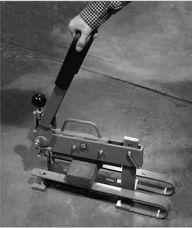
2. Then, with the handle in the "up" position, place the brick in the center of the blades underneath the Blade Hinge Pin. For accurate angle cutting, use our optional Cutting Guide Table (sold separately).
