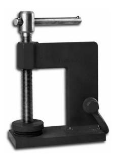
Bon stone lifting clamps are furnished with 1/2" stud in base of opening. A pilot hole drilled in the backside (unfinished side) of the stone is required for proper use. Three model sizes are available.
