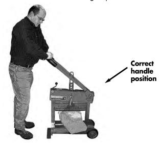
Place material to be cut in the center of the base. Lower tip blade by turning crank handle clockwise and lower handle until it rests at a  $45^{\circ}$  angle to base.
