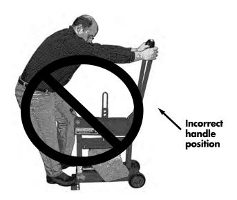
If the handle is adjusted to a position greater than 45°, the proper leverage will not be created. Press down on handle to split unit. For harder materials, it may be necessary to repeat this process. To create next cut, open handle to full open position. Turn crank handle in counter clockwise motion to raise blade. Repeat process.
