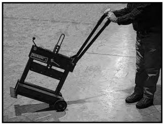
To transport unit, open handle to full open position. Insert support pin through holes at the end of the handle to lock handle in open position.
